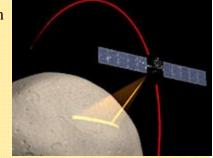
solar arrays spanning 65 feet, Dawn collects power from the sun to ionize atoms of xenon.
