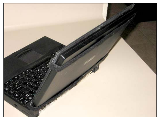
Velcro straps attach red Screen Attach Velcro to Black Plastic with Hot Glue
