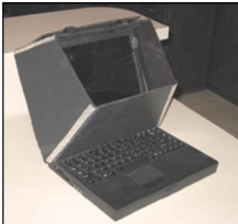
Attach flap with Velcro or tape to light shield Keep flap closed when not looking at screen
