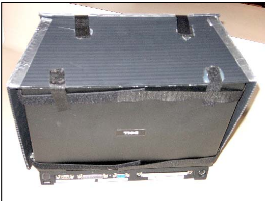
Velcro straps on light shield stick to Velcro red screen straps
