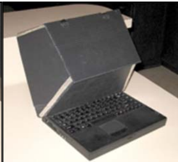
Attach flap with Velcro or tape to light shield Keep flap closed when not looking at screen
