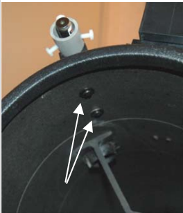
2 stainless machine screws attach pointer to the scope
