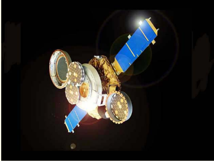
This artist's conception shows the Genesis spacecraft in collection mode, opened up to collect and store samples of solar wind particles. Credit: NASA/JPL
